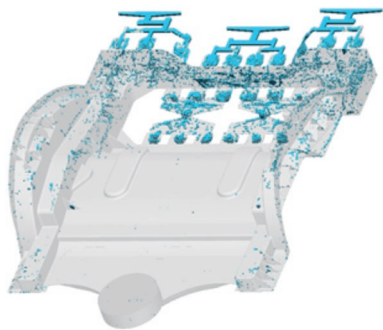
图3 Magma 软件预测的缺陷分布模拟结果 [40] Fig.3 Simulation results of defect distribution predicted by Magma software [40]
